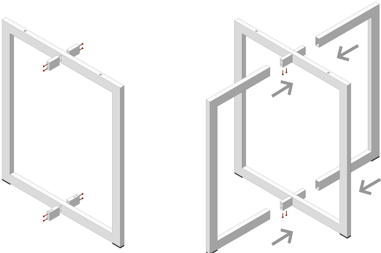
Insert element B into the two bushings and screw partially from the bottom.
